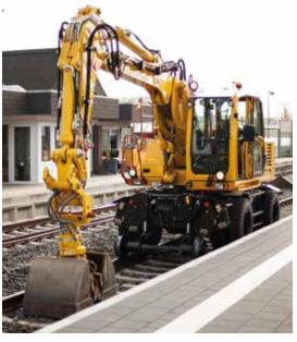
We are the sole manufacturer in Europe of rail-road, short tail swing excavators with a swing radius of less than 2000 mm in combination with the approval of German Federal Railways. We can offer any chassis configuration to fit any rail network for our world-wide customers.
