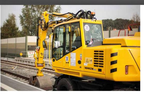
The low centre of gravity and our compact design guarantee high stability with excellent off-road mobility. 1604ZW also has a bilateral barrier on the track wheel cylinder at a swing of 5° from the longitudinal axis and at a standstill.
